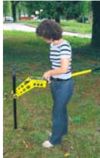
Figure 2.2: A fluxgate magnetometer. The two sensors of the gradiometer are mounted at opposite ends of the vertical black tube.
